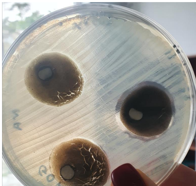
Fig. 11. inhibition zone of a test culture on rGO-AgNps
