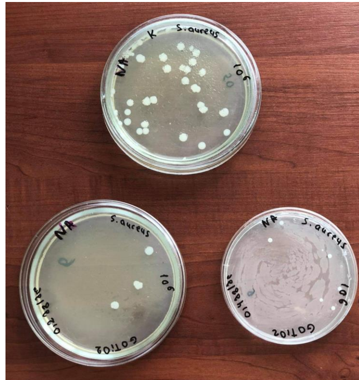
Fig. 15. viable cell count of test culture on rGO-TiO 2
