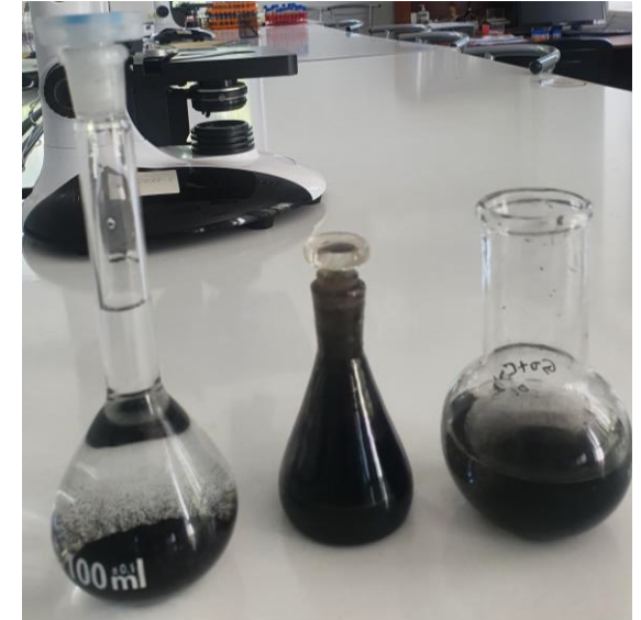
Fig. 11. Homogenized nanoparticles of TiO 2 , Ag, Cu
