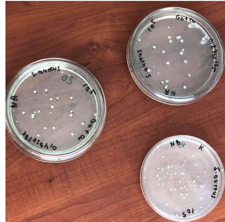
Fig. 14. viable cell count of test culture on rGO-Cu
