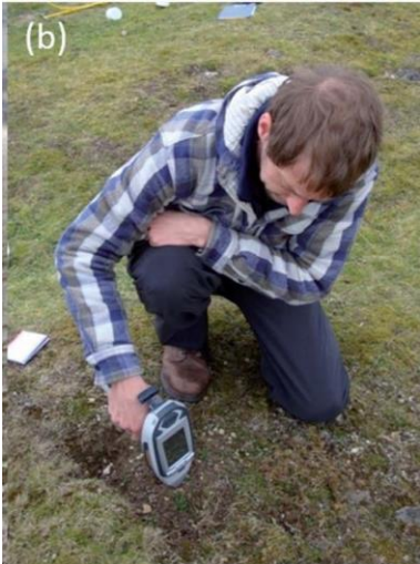
hand-held portable X-ray Fluorescence (pXRF) on soil at 5 mm scale
