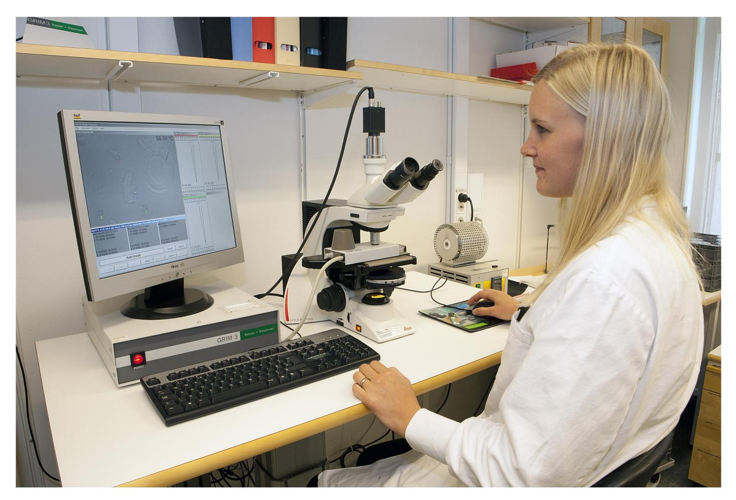
One of the methods used in forensic glass analyses is to measure and to compare refractive indices. The instrument used for these measurements is GRIM 3 (Foster & Freeman Ltd), see figure 1. A control chart is used as an internal quality control for these measurements, see figure 2.
