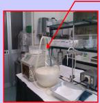
In the phase of dispensing two peristaltic pumps were used (one for milk dispensing and the other for maintaining the homogenization of the bulk material)
