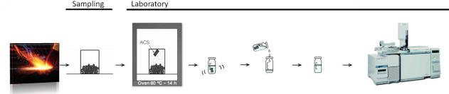
Identification and data analysis by GC-MS - ASTM E 1618-10
